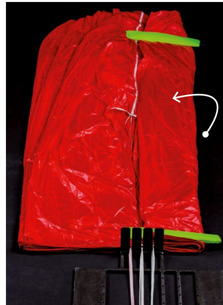
Double over the right canopy half towards the centre axis.
