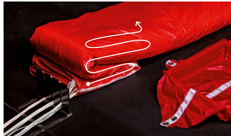
Fold the canopy in an S-shape to 90% of the deployment bag length. You will need the remaining space for the suspension lines.
